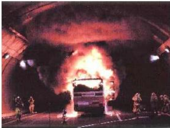
Figure 7-10 Tunnel Fire Test
